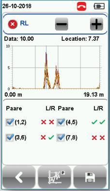
Return Loss failed because cable was run over and crushed by forklift truck after approx. 7m
